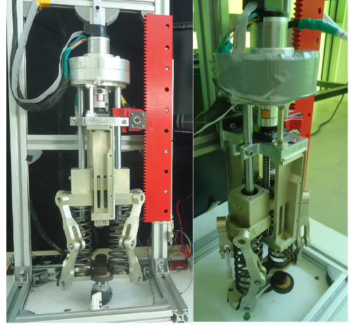
Figure 1: Vertically constrained hopper platform with series elastic actuation.
